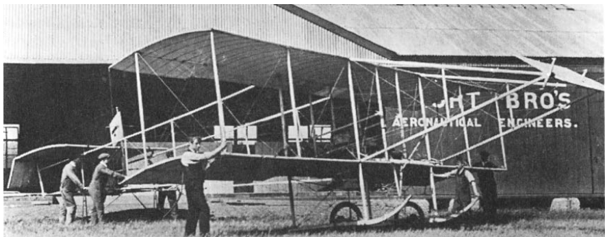
Designed by Horace Short and based on the successful Farman III pusher biplane, the Short S27 was the principal training aircraft in the early days at Eastchurch.
