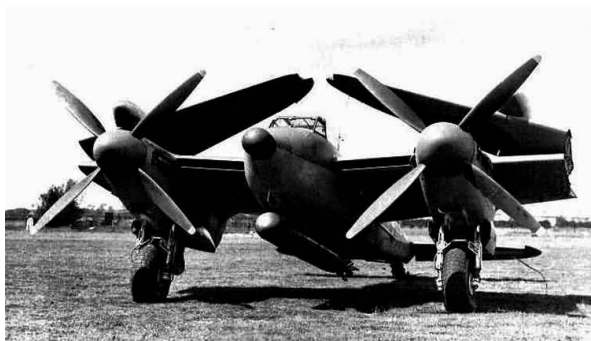
The Sea Mosquito with wings folded. Note the "thimble" radome. Although shown loaded with a torpedo, the Sea Mosquito did not see front line service.
