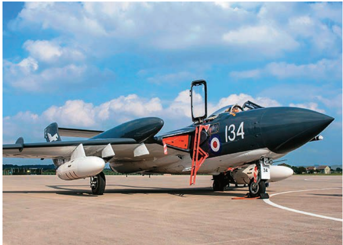
Sea Vixen at rest. The "frangible" hatch over the observer's cockpit is open
