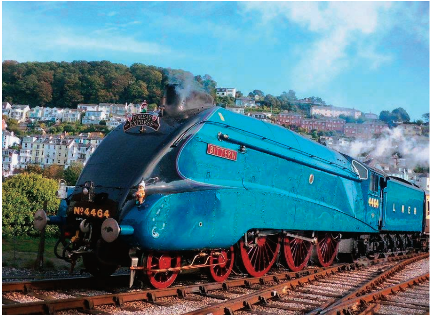
"Bittern" is a Pacific 4-6-2 locomotive, built to the same design by Sir Nigel Gresley as the more famous A4 "Mallard", holder of the world speed record for steam locomotives. Photo R Hufton
