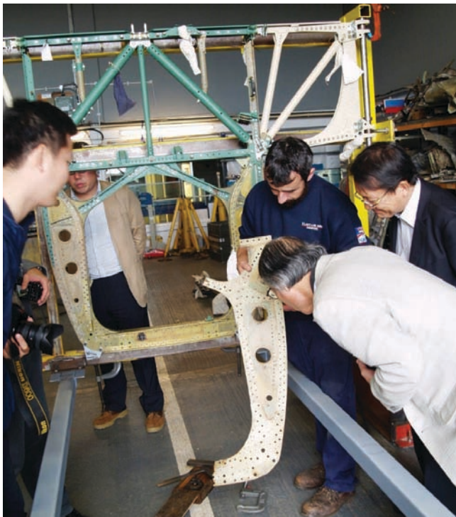
Museum Restoration Engineer William Gibbs showing the Japanese Institute delegates details of the Barracuda restoration, and how he is re-incorporating as much original Barracuda material as possible back into the rebuild.
