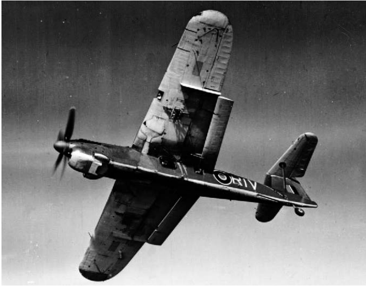
Not a beautiful aircraft - Barracuda Mk 2 in flight. The high-set tailplane and distinctive Fairey Youngman flaps-cum-dive brakes can be clearly seen
