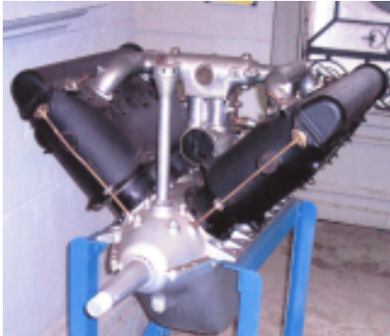
The direct drive Hispano-Suiza 4 series engine, licence-built by Wolsley Motors
