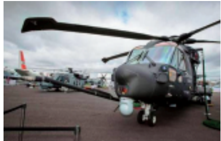
“What a long nose you have!” The US-style retractable In-Flight Refuelling (IFR) probe
