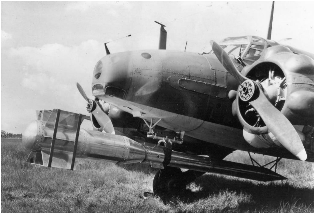
Above; An Avro Anson of the N.A.R.I.U. assisting with trials of the Liquid Oxygen-Petrol, Guided Anti-Aircraft Projectile, (LOPGAAP) which was suspended backwards on the bracket used to hold the ASH radar, for telemetry tests, at RAF Christchurch in May 1945.
