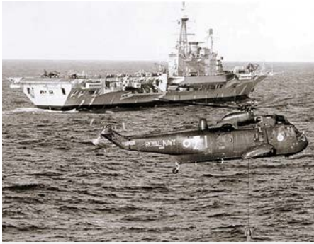
Sea King HAS.1, XV672/71/H of 814 NAS demonstrates its SONAR dipping capability for the camera with HMS Hermes (R12) in the background. © Royal Navy
