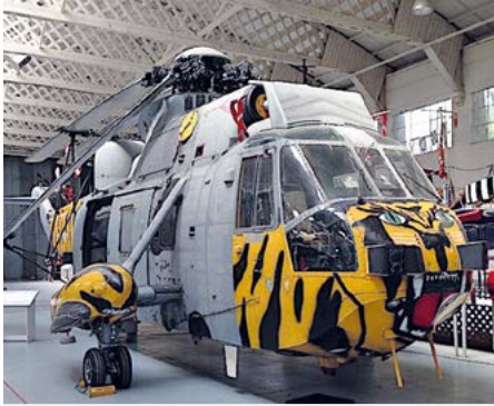
Originally built as a Sea King HAS Mk.1 - first flight on 8 March 1972 - this airframe eventually went back to Westland in 1987, and upgraded to HAS Mk.5 specifications, and then again in 2000, to be upgraded to HAS Mk.6 specifications. This long serving Sea King was finally retired in 2010, and placed in the collection at the Imperial War Museum (IWM). It is seen here at IWM Duxford in the colours of its last operational Royal Navy squadron, 814 Naval Air Squadron. © MoD
